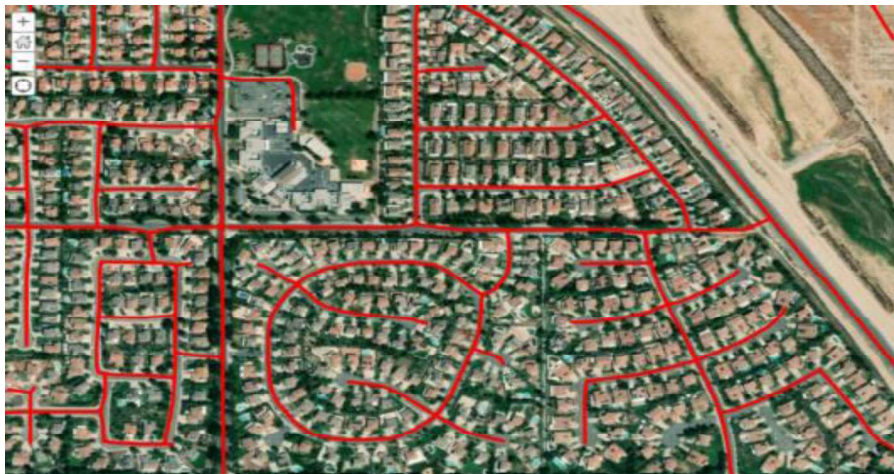
Figure (4): Roads detected using deep learning and converted to geographical features (Nassar et al, 2023)
